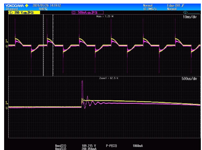
Figure 3 LED Driver Inrush Current on Triac Dimmer
