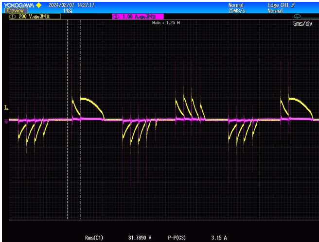
Figure 4 Triac Dimmer Holding Current
