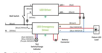
For additional wiring diagrams please visit <u>https://www.hatchlighting.com/elp-alternate-wiring-diagrams</u>
