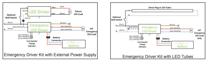
For non-LED fixtures, please use "Emergency Driver Kit with External Power Supply" wiring diagram.
